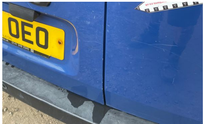
4: Door osf Dented Over 30mm
