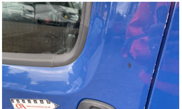
6: Tailgate Dented With Paint Damage
