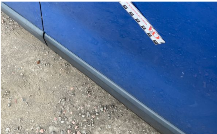
5: Sill os Poor Previous Repair Paint Flake
