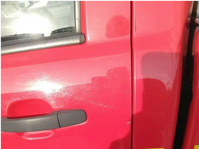
5: Door nsf Chipped Edge Chip
