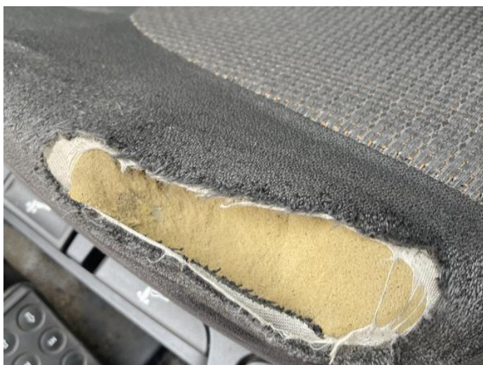
1: Seat Base Cover osf Torn Over 3mm
