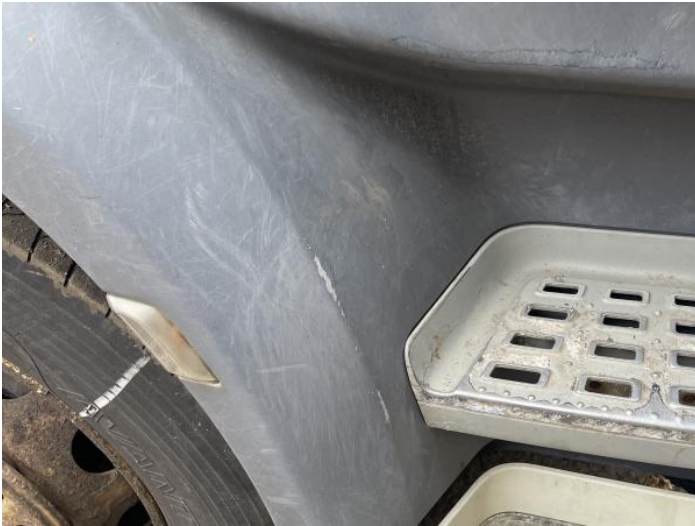
3: Door Moulding osf Scuffed (Unpainted) Over 100mm
