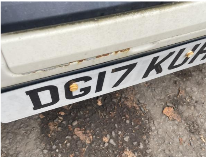
5: Bumper Front Rusted Over 5mm
