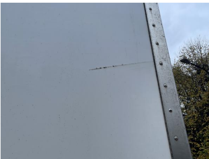
7: Qtr Panel nsr Dented Over 30mm
