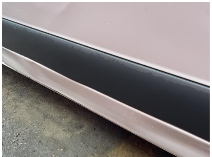
8: Door nsr Dented Over 30mm
