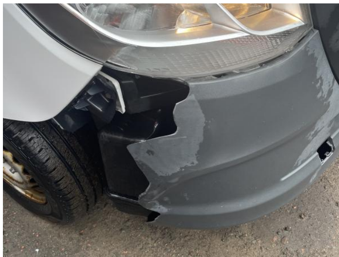
2: Bumper Front Moulding Broken Replace
