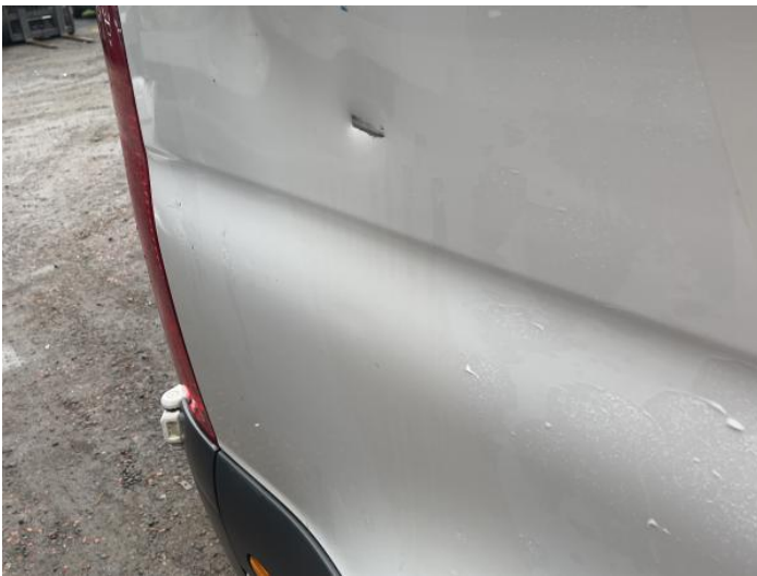
5: Qtr Panel osr Dented With Paint Damage
