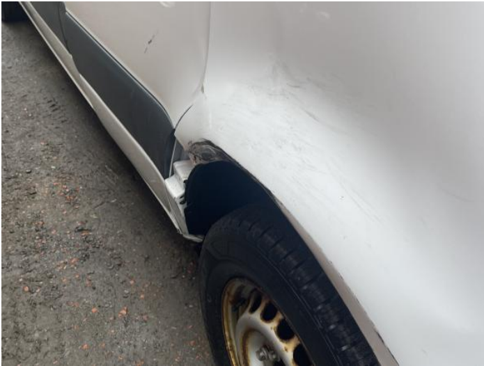
3: Wing nsf Dented With Paint Damage
