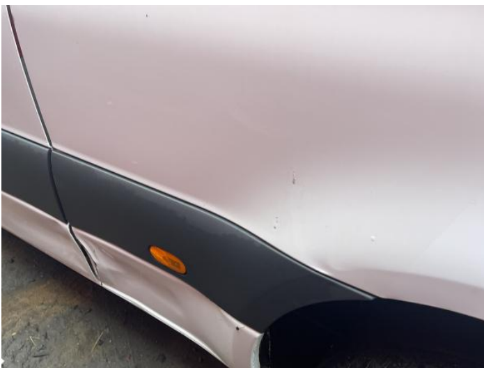
7: Qtr Panel nsr Dented With Paint Damage
